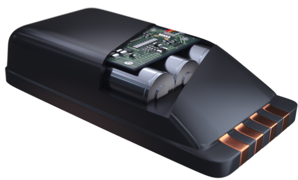
ILLUSTRATION OF BATTERY MANAGEMENT SYSTEM SHOWING CIRCUIT BOARD AND BATTERIES.
