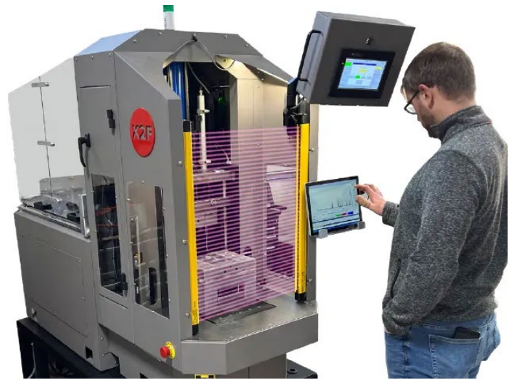
Colorado-based X2F developed its own molding machine to use its patented Controlled Viscosity Molding process. The system's very low pressures make it safer to overmold materials onto highly sensitive electronics. Image courtesy of X2F.
